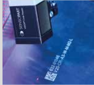
Lasered code on shiny metallic surfaces
